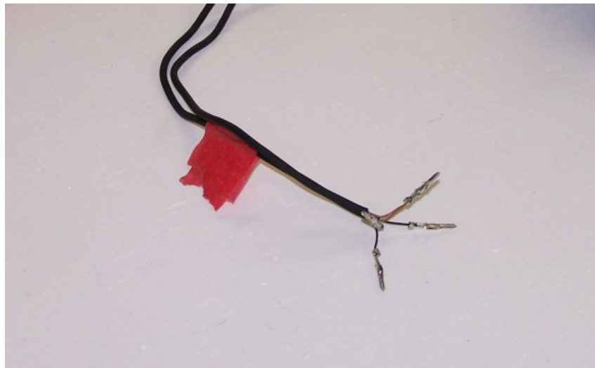
Installed Crimp Pins
